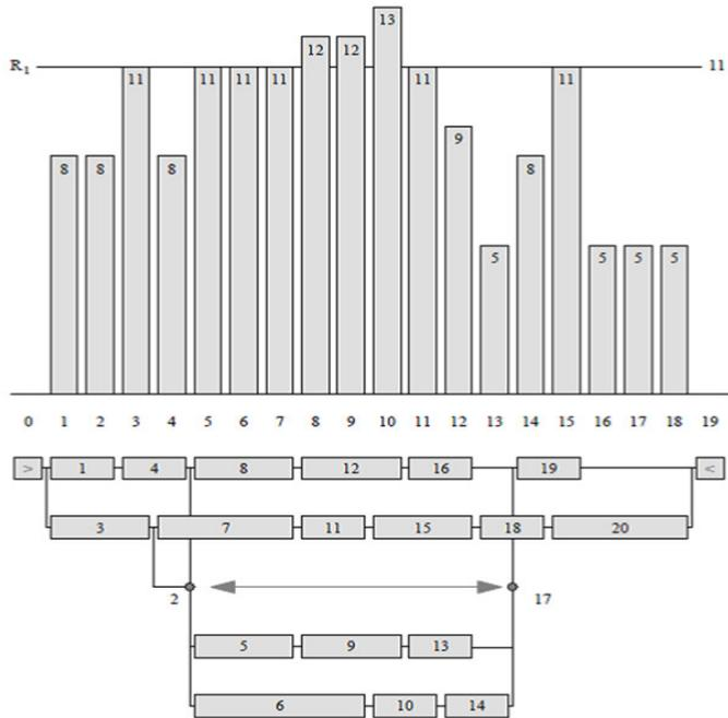
**Figure 3: The early CPM of a simple example (Csébfalvi G. and Csébfalvi A., 2005)**
